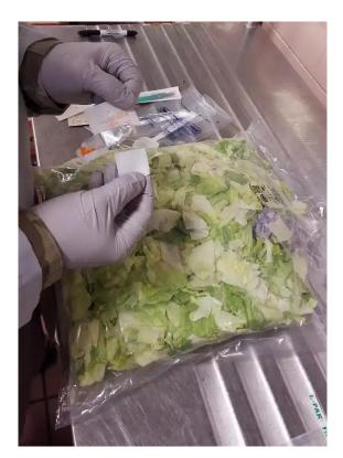
Select an area of the package that can be easily decontaminated. This area must be large enough to remove sample. Taking an alcohol pad, start in the center of the selected area and wipe in a circular motion to just outside the area that will be cut open.
