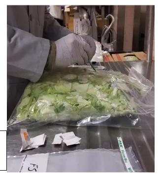
Using a sterile scalpel blade, cut a flap in the area of packaging that was decontaminated.
